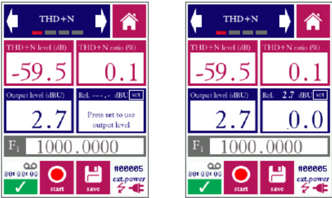
Measuring screen before setting a reference level (left) and after setting the reference level in dBU to 2.7 dB (right)
