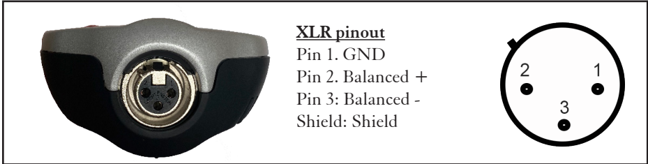
Top of the device: XLR connector.
