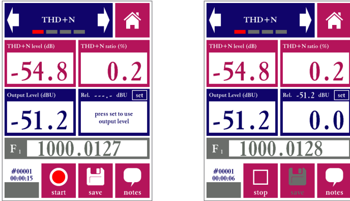
Measuring screen before setting a reference level (left) and after setting the reference level in dBu to 2.7 dB (right)
