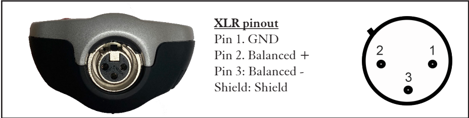
Top of the device: XLR connector.
